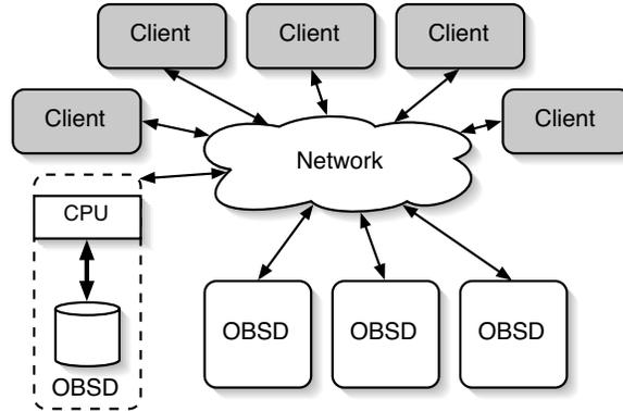
Figure 1: A typical NASD-based storage system
