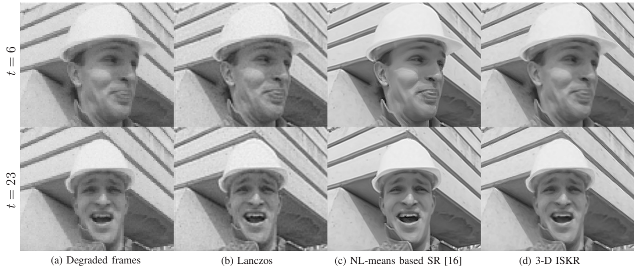
Fig. 10. A video upscaling example using Foreman sequence: (a) the degraded frames, (b) the upscaled frames by Lanczos interpolation (PSNR: 31.01 (top) and 30.21 (bottom)), (c) the upscaled frames by NL-means based SR [16] (PSNR: 32.13 (top) and 31.94 (bottom)), and (d) the upscaled frames by 3-D ISKR (PSNR: 33.02 (top) and 32.12 (bottom)). Also the PSNR values for all the frames are shown in Fig. 12(c)
