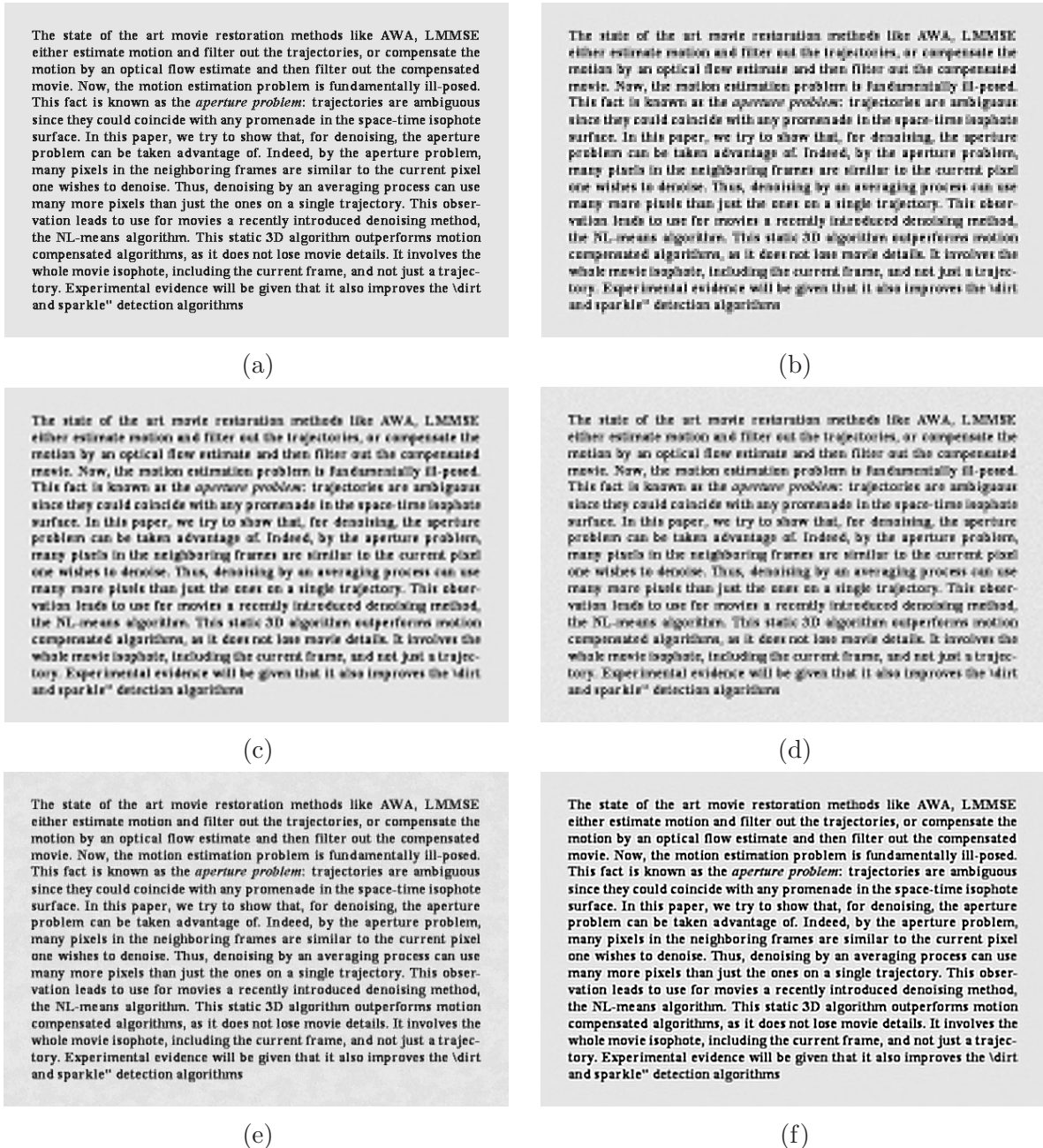
Figure 6: Results for the synthetic text sequence. (a) Original (ground-truth) image. (b) Pixel replicated image, 13.47dB. (c) Lanczos interpolation, 13.84dB. (d) Deblurred Lanczos interpolation, 13.9dB. (e) Result of shift-and-add algorithm [18, 20], 18.4dB. (f) Result of proposed algorithm, 18.48dB.
