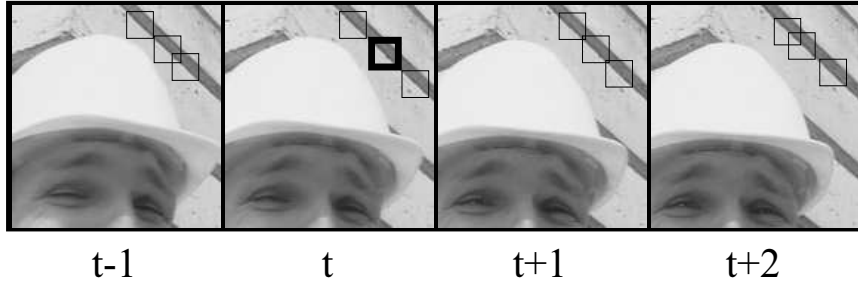
Figure 3: NLM’s fuzzy motion estimation: A patch in the reference image at time t (marked with a thick line) has several probable locations in the other images, and also within the same image itself (marked with narrow lines).
