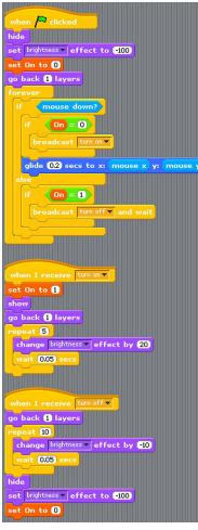
Flashlight 1 uses one script to do all the interaction with the mouse. It has a variable to keep track of whether the light is on or not, and sends broadcast messages to turn the light on when the mouse is pressed and the light is off, and to turn the light off when the mouse is pressed and the light is on. Separate scripts turn the light on slowly or off slowly.
