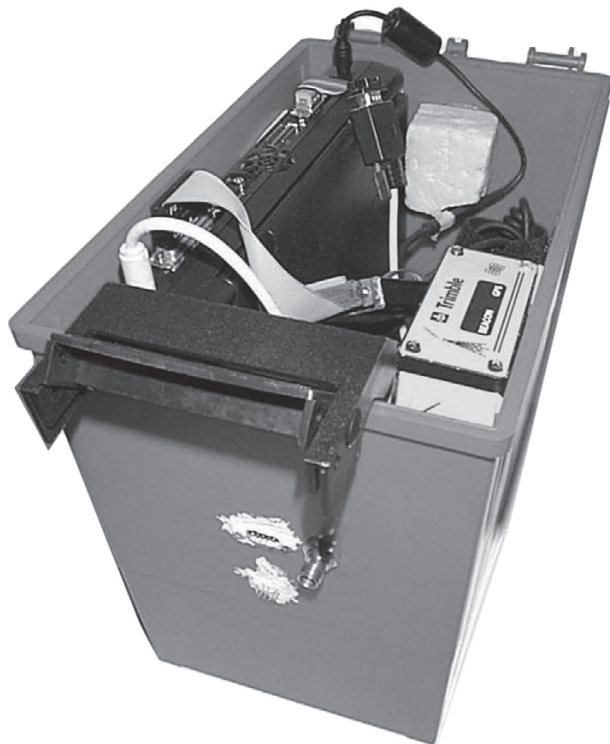
Fig. 5—Guidance, Navigation, and Control computer box, with the Trimble Ag122 DGPS Receiver, A Pentium Class laptop, and DC-DC converter to power the laptop, and an ESD Parallel port CAN dongle. The entire box is sealed and has water-tight connections for Power, CAN, and the RF signal from the GPS antenna.
