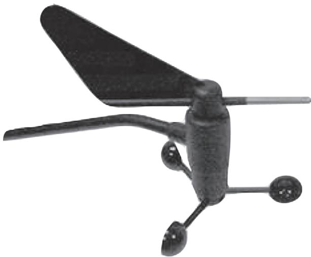
Fig. 8—A 3-cup anemometer is used to determine wind speed and direction. The unit is made by Standard Communications Electronics, and has a two-pulse per revolution output for the cups, and a quadrature analog signal for the direction of the weathervane. It was calibrated in a wind tunnel.
