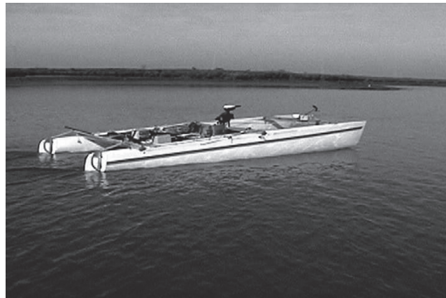
Fig. 12—The Atlantis on an unmanned trajectory being controlled by the identified LQG controller. Propulsion is from a MinKota trolling motor running at 12, 24, and 36 Volts. The motor is canted off the center line to simulate off-center thrust as would be seen by the wing-sail.
