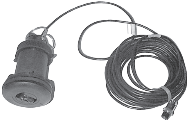
Fig. 7—Hullspeed sensor is located towards the rear of the starboard hull, and is made by the Standard Communications Electronics Corporation. Due to its location behind the centerboard of the hull, the signal is quite noisy from the turbulence.
