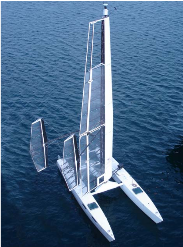
Figure 1. HWT X-1 Prototype vehicle, as viewed from above. The vehicle is based on a modified Stiletto 27 Catamaran.
