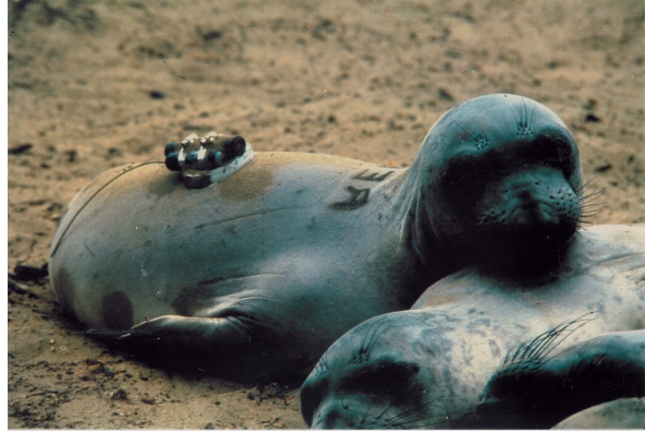
Fig. 2. A young elephant seal with a modern time data recorder (TDR) affixed to its body. This TDR is approximately 4 times as large as the prototype MAMMARK tag.
