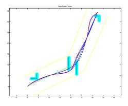
Fig. 3. We iteratively generate smooth curves(blue) bending them around obstacles until a collision free path(red) is found.
