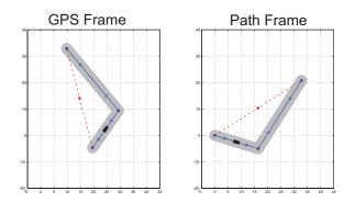
Fig. 1. The current waypoints (blue) and corridor (grey) must be rotated to guarantee that the points are monotonic.
