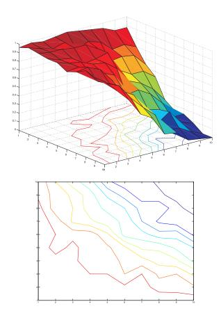
Fig. 4. Monte Carlo simulations were run over environments having between 5 and 50 obstacles of size up to several square meters to determine the success rate of the algorithm.
