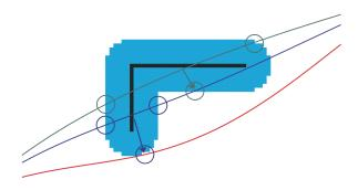
Fig. 2. The midpoint of the collision is moved out until a clear path is found.
