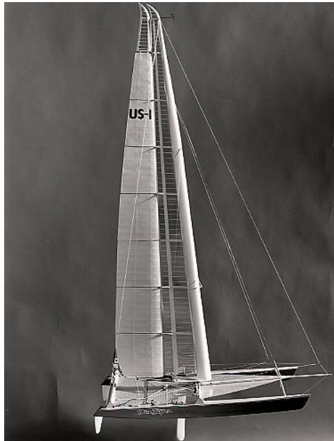
Figure 1-14 The wingsailed catamaran Stars and Stripes . This catamaran was built to answer a poorly framed challenge for the America's Cup race in 1988. The wing was designed by Jon Roncz and built by Burt Rutan. The Stars and Stripes won the 1988 America's Cup easily, but both captain and crew were never entirely comfortable sailing her. The wing was fixed as opposed to self-trimming, and was very mechanically complicated.
