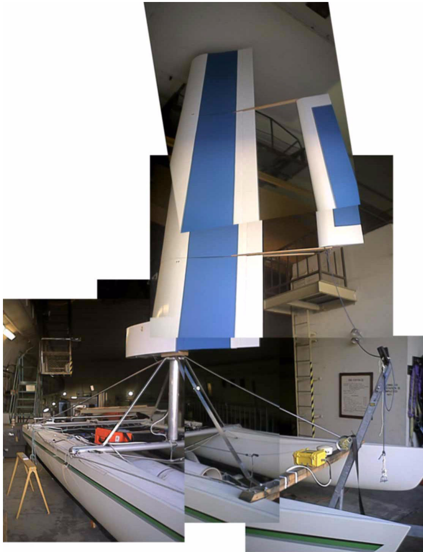
Figure 5-52 Final Atlantis wing, with spider below and electronics pod. This is a composite image made up of several photographs of the Atlantis taken inside the HEPL high bay entrance. The entire system was assembled inside of a hangar in order to perform a final system check before performing the water trials. The clearance between the top of the wingsail and the roof of the hangar is approximately 12 cm.
