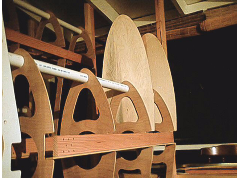
Figure 5-45 Main wing ribs on jib, spar caps, and pod ribs extending forward on lower wing section. The forward pod ribs are double thickness plywood, and the PVC pipe spacers ensure uniformity in the rib spacing. The spar caps are glued in place with epoxy. The top of the spar caps has been drilled for the aluminum mortise and tenon joint that holds the wing sections together. The three sections will be held together with stainless steel bolts at the joints.
