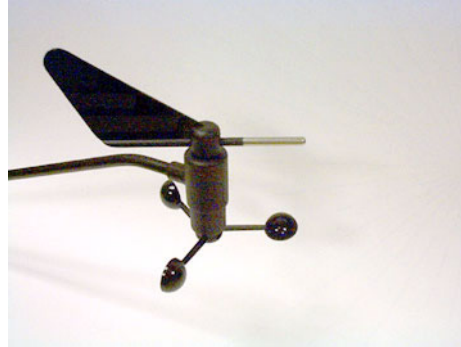
Figure 2-5 Standard Marine Electronics anemometer and weathervane transducer. The weathervane outputs an analog quadrature signal with a 5 volt sine and cosine components. It is capable of recording absolute position of the weathervane from 0 to 360 degrees without wind-up. The anemometer produces a square wave proportional to the wind speed. The greater the frequency of the square wave, the greater the wind speed.
