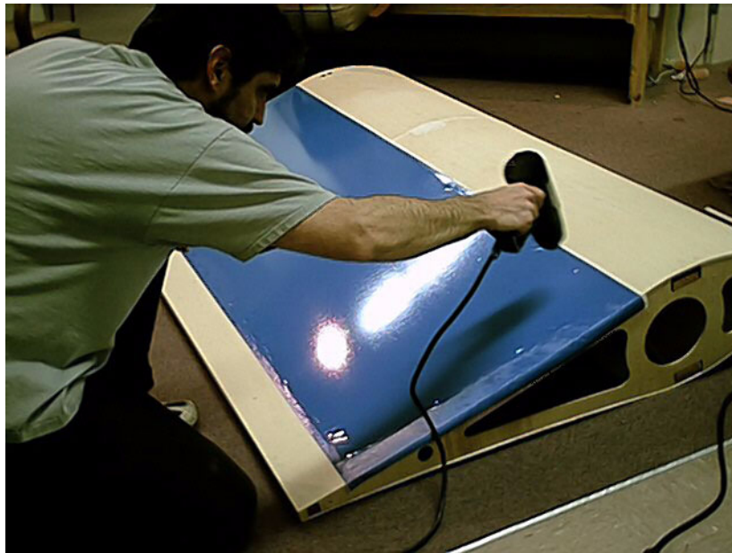
Figure 5-49 Coverite polyester fabric is used to cover the wooden wing structure. Cris Hawkins of Cris Hawkins consulting applies heat to shrink the fabric onto the ribs. The covering is oil, gasoline, and salt-water resistant. In order to prevent the fabric from pulling off the ribs on the rear section of the airfoil, the fabric was glued down to the ribs during the shrinking process through a process of applying pressure while the coverite was allowed to cool.
