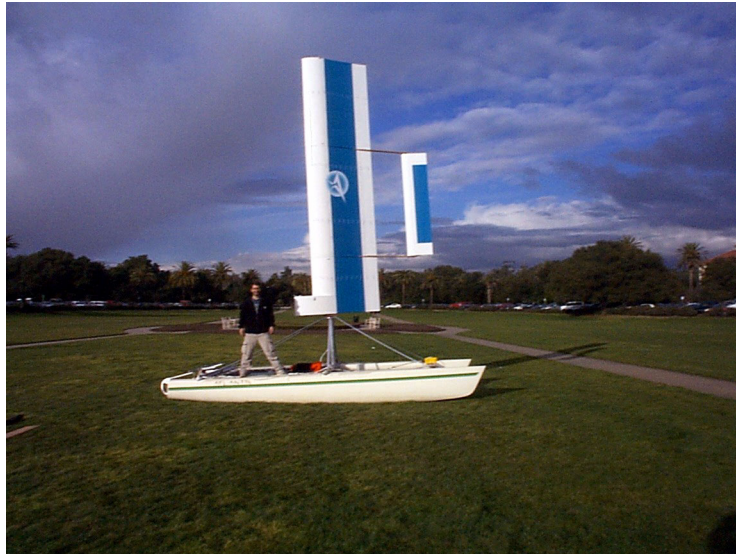
Figure 2-1 The Atlantis, assembled on the Stanford Oval. The hulls and crossbeams are originally from a Prindle-19 day-sailing catamaran. The author is included in the picture to give a sense of scale. The wing is free to pivot on bearings and is trimmed by aerodynamic loads on the fully flying tail.
