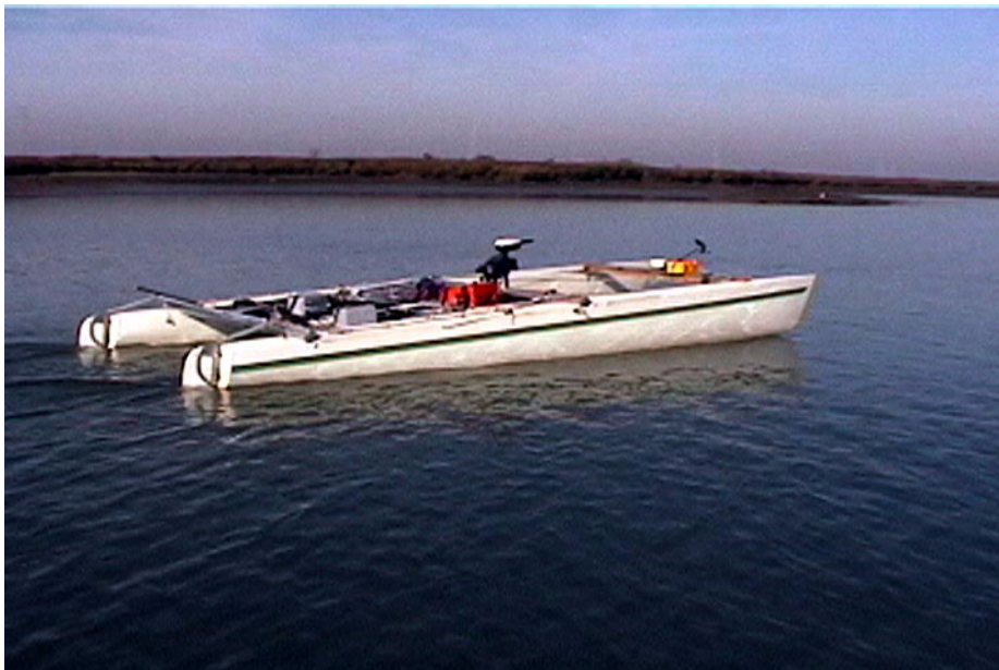
Figure 3-12 The Atlantis propelled by a trolling motor, as setup for hullspeed calibration. A series of measurements were made using the GPS velocity to calibrate the hullspeed sensor. It was found that the rudder angle had a very large impact on the hullspeed reading (the aforementioned coupling), and thus the calibrated hullspeed equations use both the rudder angle and raw hullspeed sensor measurements as inputs.
