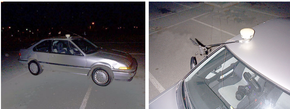
Figure 3-6 Acura Integra with anemometer and GPS antenna installed for experimental validation of the linear calibration of the anemometer. Velocity was recorded from GPS, and from the anemometer as well. Flow effects due to the shape of the car, as well as any ambient wind, will distort the measured airspeed. Tests were performed on calm nights to minimize the ambient wind.
