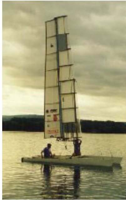
Figure 1-15 Cornell RAFT project was an undergraduate effort to build a high performance wing for a catamaran. The wing uses carbon fiber ribs with a mylar covering to achieve light weight. The wing is asymmetrical, with a leading edge slot and a trailing edge flap. The wing is tacked “over-the-top” by pivoting the aft section at the vertical center behind the leading edge slat section.
