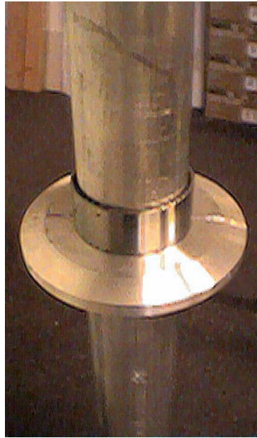
Figure 5-40 Stub mast, inner bearing surface for needle roller bearing, and stub mast collar for attachment of the aluminum spider. The lower needle roller bearings roll on the surface just above the collar. The collar is used to secure the 6061 aluminum straps (instead of stainless steel guy wires) that support the stub-mast and wing.
