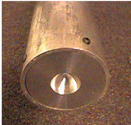
Figure 5-42 Stub mast seat that mates with teflon hemisphere on catamaran forward crossbeam. The stub-mast seat was machined out of 6061 aluminum, and is held into the stub-mast by four stainless steel 5/16" machine screws. This allows the easy removal of the stub-mast from the catamaran.
