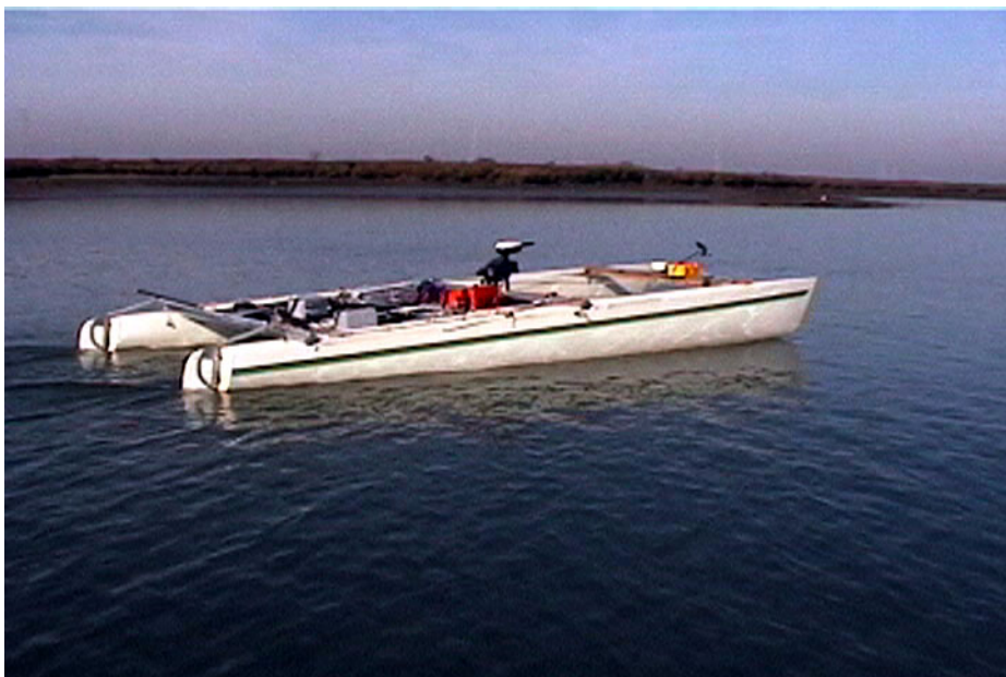
Figure 7-7 The Atlantis unmanned trolling motor test run. The trolling motor is canted off the centerline in order to simulate the presence of a wing sail and all steering control is through the control system.
