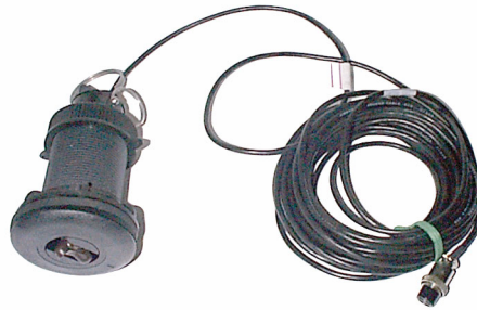
Figure 2-6 Standard Communications Electronics hullspeed sensor, pictured before installation on starboard hull. This through hull sensor remains semi-submerged in the flow of the water around the hull. It has a magnetic four-armed paddle wheel and a Hall-effect sensor to produce a square wave whose frequency is proportional to the velocity of the water flowing past the sensor (or the velocity of the sensor through the water).
