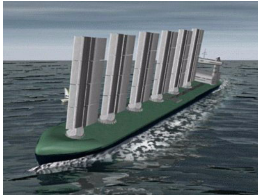
Figure 1-17 The Dutch Pelmatic wingsailed oil tanker proposal. This oil tanker is to use five independent wingsails that are tacked by splitting each wing into four vertical sections that independently rotate about the mast in an over the top fashion. The design includes two 50' deep swing keels to make sailing efficient. The wingsails are expected to reduce fuel consumption by over 50%.
