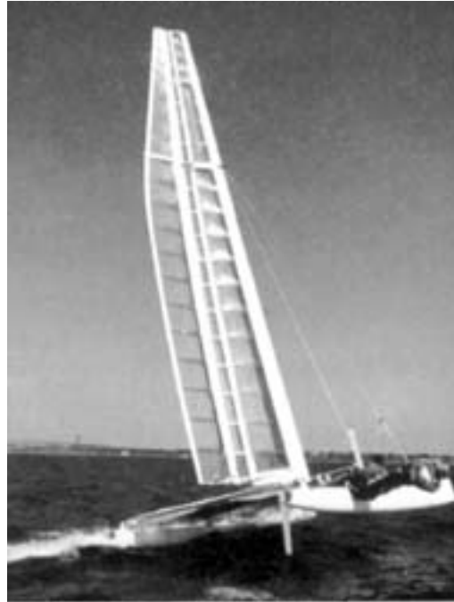
Figure 1-9 Ms. Nylex , winged Class “C” catamaran, built in 1972. She raced and won the “Little America’s Cup” in 1972. The wing has a simple NACA 0015 section, but with a large 60% trailing edge flap. The wing was trimmed conventionally, with the usual assortment of winches, pulleys, and lines. The ability to trim the top and bottom of the wing separately, effectively managing the twist of the wing, was considered crucial to the victory.
