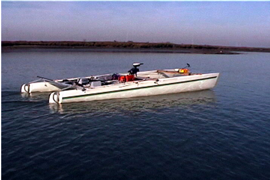
Figure 6-12 The Atlantis on the water with the trolling motor and extra batteries for ballast. This was the configuration of the Atlantis when taking data for OKID identification.
