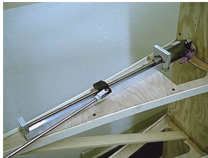
Figure 2-12 A view of the installed flap actuator in the lower wing section before covering. The flap and tail actuators are identical. The actuators are Pitman 24V DC motors, de-rated to 12V. A stainless steel lead screw assembly is used to move a delrin macpherson nut. Stainless steel pushrods are attached to the macpherson nut, which are connected to control horns (not shown) on the flaps and tail.
