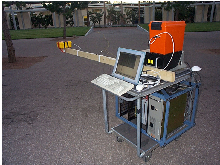
Figure 4-14 Experimental setup to validate magnetometer calibration algorithm. The yellow box at the end of the wooden boom contains the Honeywell HMR-2003 three-axis magnetometers and a microcontroller. It was placed out at the end of the wooden boom to minimize the effect of the magnetic fields of the INS power supply located beneath the orange box. Data was taken by pitching, rolling, and yawing the entire setup repeatedly.
