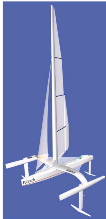
Figure 1-18 An artist rendition of the Volantis , an 80 feet long foil borne trimaran with a rigid self-trimming wing sail that includes a cloth jib. It is intended to set a new Pacific crossing speed record, and also to be used to tow microphone arrays in an autonomous mode. This is a commercial project with preliminary funding. They have not yet built a prototype.
