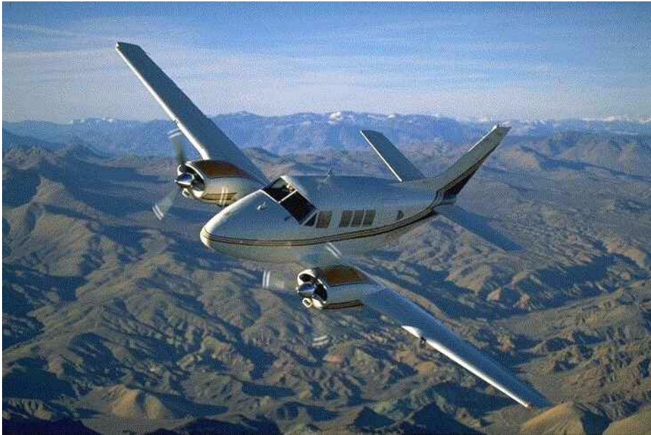
Figure 4-18 Beechcraft/Raytheon QueenAir used for experimental testing of attitude algorithm. This aircraft is equipped with a short baseline GPS attitude system, a Honeywell HMC-2300 digital three-axis magnetometer, Crossbow DME-FOG, and a navigation grade INS. The aircraft was instrumented using the gyroscope-free quaternion attitude estimator and flown through various steep turns. The attitude was found to be in excellent agreement with the INS.
