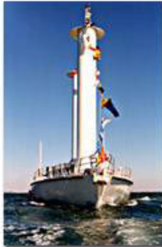
Figure 1-13 The Cousteau Society turbosailed vessel Calypso II uses a modern version of the Magnus rotor. Instead of spinning the cylinders to provide lift, turbosails suck the boundary layer off with vacuum pumps through a porous surface. In addition, a movable flap is used to effectively “tack” the turbosails.
