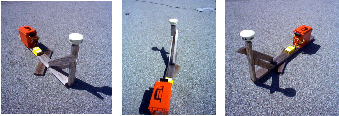
Figure 3-21 The GPS dynamic spin rig. This spin rig was used to test the GPS position performance under dynamic conditions. The spin rig is a merry-go-round, balanced on a lazy susan bearing. The yellow box is the receiver, and the white object on the post the antenna. The entire system is battery powered, obviating the need for slip rings. The rig was spun by hand, attempting to keep a steady angular rate of one revolution every 5-7 seconds.
