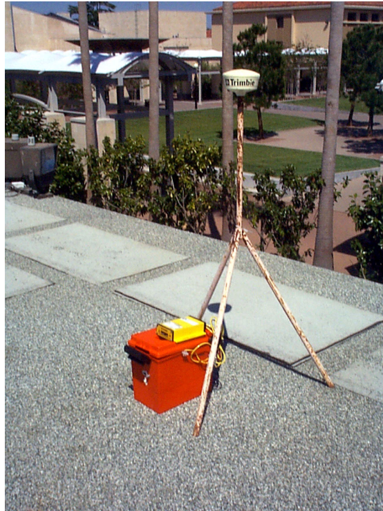
Figure 3-20 GPS setup for static test. The GPS receiver was located on the roof of a building on Stanford University campus. The roof was chosen to be above the surrounding buildings in order to minimize the possibility of multipath errors. Data was recorded once per second for 24 hours. This was used to determine the static position statistics for this GPS receiver.
