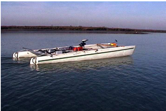
Fig. 5. The Atlantis on an unmanned trajectory being controlled by the identified LQG controller.
