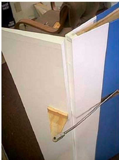
Figure 5-50 main wing trailing edge flap with pushrod, control horn, and fabric hinge. The figure 8 hinge is made from the same covering material that covers the wing. The advantage of this kind of hinge is that there is very little hinge friction. Additionally, the hinge seals the gap between the flap and main section, while at the same time allowing a large range of motion.
