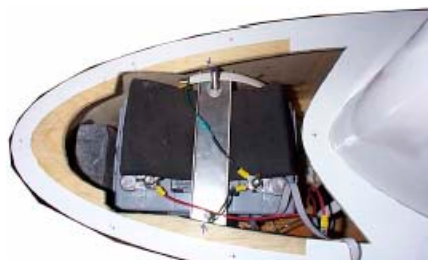
Figure 5-51 Electronics pod, showing the battery and ballast weight. Inside the pod is the main battery, secured by two threaded stainless steel rods. The black material is neoprene for cushioning the electronics. Forward of the battery is a 12.7 kg lead brick that is used to mass balance the wing. The wires lead to the main bus breaker on the side of the electronics pod. The ribbon cable joins the can bus and the anemometer microcontroller which is secured to the underside of the pod lid.
