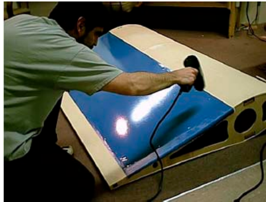
Figure 5-49 Coverite polyester fabric is used to cover the wooden wing structure. Cris Hawkins of Cris Hawkins consulting applies heat to shrink the fabric onto the ribs. The covering is oil, gasoline, and salt-water resistant. In order to prevent the fabric from pulling off the ribs on the rear section of the airfoil, the fabric was glued down to the ribs during the shrinking process through a process of applying pressure while the coverite was allowed to cool.
