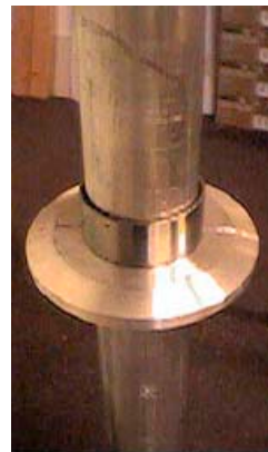
Figure 5-40 Stub mast, inner bearing surface for needle roller bearing, and stub mast collar for attachment of the aluminum spider. The lower needle roller bearings roll on the surface just above the collar. The collar is used to secure the 6061 aluminum straps (instead of stainless steel guy wires) that support the stub-mast and wing.
