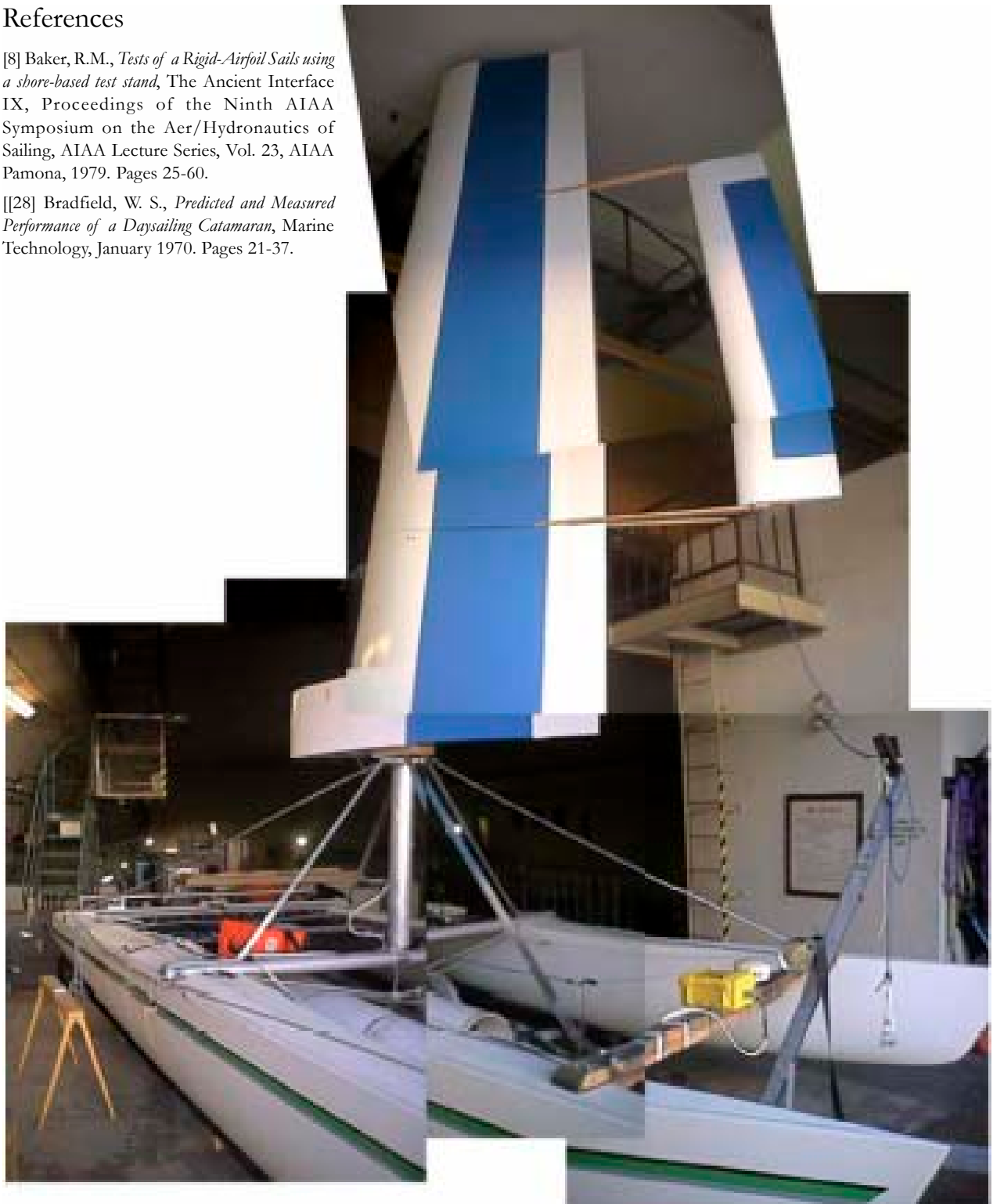
Figure 5-52 Final Atlantis wing, with spider below and electronics pod. This is a composite image made up of several photographs of the Atlantis taken inside the HEPL high bay entrance. The entire system was assembled inside of a hangar in order to perform a final system check before performing the water trials. The clearance between the top of the wingsail and the roof of the hangar is approximately 12 cm
