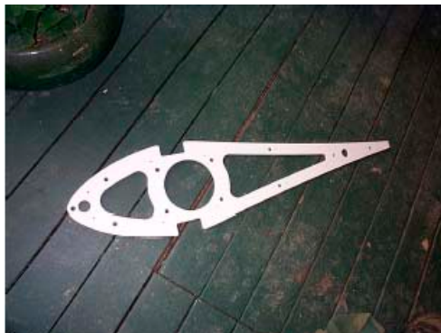
Figure 5-44 Master main wing rib template used to fabricate all wing ribs from marine grade plywood. The large holes are to lighten the ribs. The two medium sized holes forward and back are for a assembly onto a jib made of electrical conduit. The eleven small holes are for threaded rods that secure the stack of plywood together to ensure uniform fabrication.
