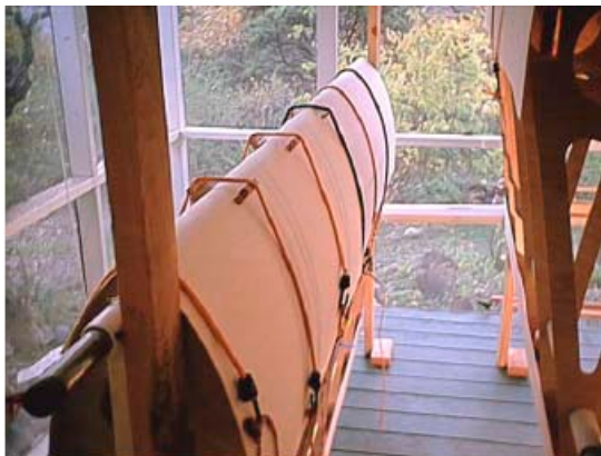
Figure 5-46 Plywood leading edge skin glued to wing ribs. The wing skins suffered severe cracking problems when bent around the leading edge. In order to accommodate the sharp radius of curvature, the wing skins were thinned and soaked in water before gluing them on to the ribs to form the forward “D” tube. This area remained weak and prone to damage in the finished wing structure.
