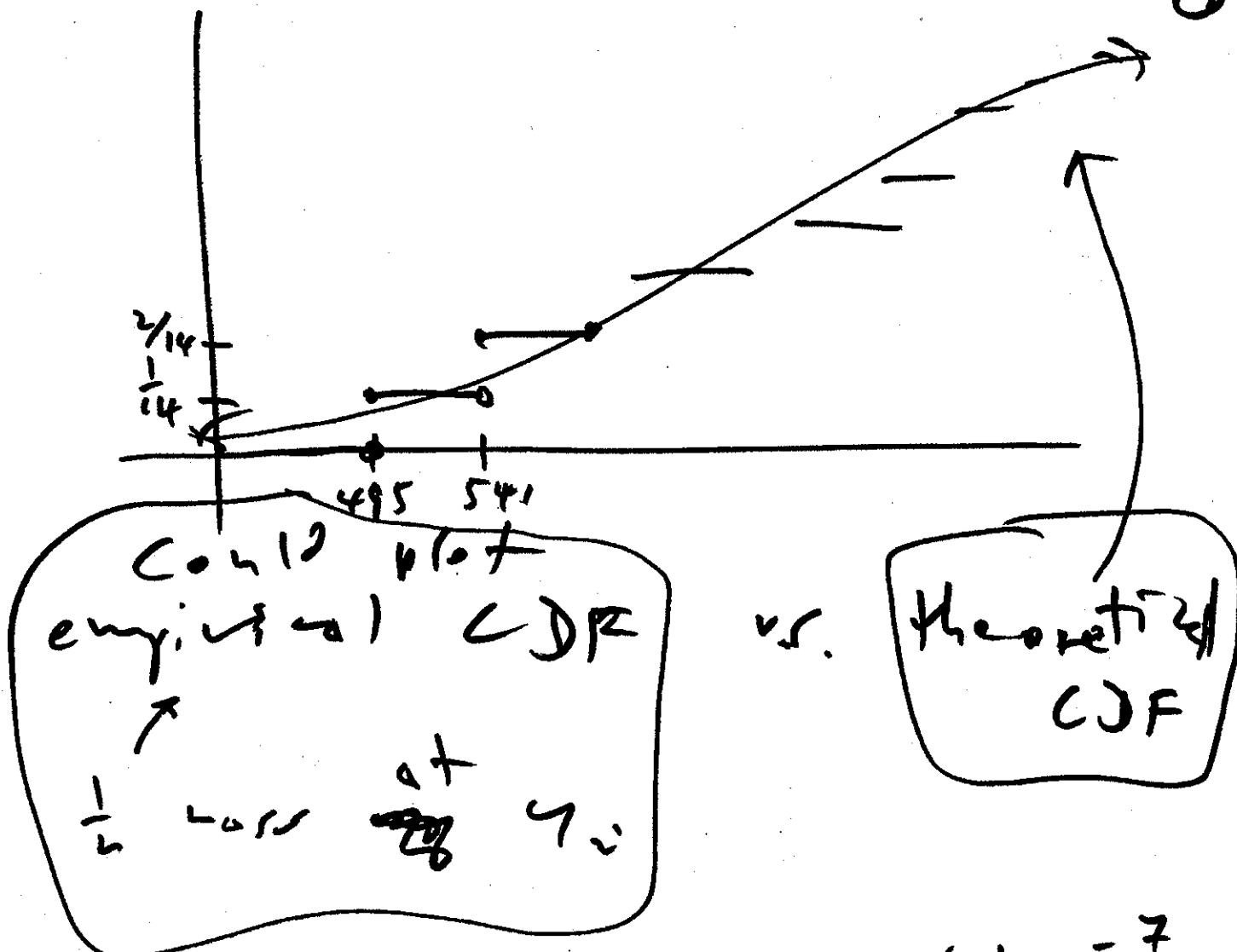
$$\Omega \sim \mathcal{E}(\gamma) \quad p_{\Omega}(y|\gamma) = \begin{cases} \frac{1}{\gamma} e^{-\frac{y}{\gamma}} & \text{for } y > 0 \\ 0 & \text{else} \end{cases}$$
