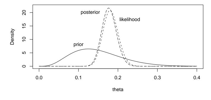
Then the **prior** is Beta(4.5, 25.5), the **likelihood** is Beta(73, 329), the **posterior** for  $\theta$  is Beta(76.5, 353.5), and the three densities plotted **on the same graph** are given above.
