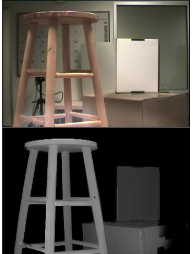
Figure 2: An example of a depth image produced by an SLP sensor. Far objects are shaded with increasingly darker tones of grey.
