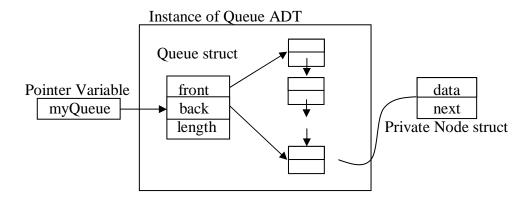
Two more C functions are necessary. One to create new objects (constructor) and one to free memory associated with ADT instances no longer in use (destructor). It is the responsibility of these functions to manage all of the memory inside the 'black box', balancing calls to malloc (or calloc) and free.
