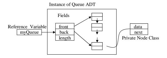
The user of the ADT should never be allowed to directly access the 'structure' inside the 'box'. Instead a reference variable (myQueue) points to an instance of the class and is passed as an (implicit) first argument to the methods of the class. For example, the call
