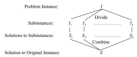
To say that the subinstances are solved recursively means that the same divide and conquer technique is applied to each of them, obtaining yet smaller instances of the problem. This process eventually reaches a point where the size of the problem instance is so small, that the solution is trivial.
