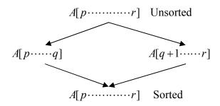
Merge(A, p, q, r) requires as precondition that the subarrays  $A[p\cdots q]$  and  $A[q+1\cdots r]$  are already sorted, and that  $p \le q < r$ . It copies each subarray into temporary spaces  $T[p\cdots q]$  and  $T[q+1\cdots r]$ , then steps through the temporaries from left to right, comparing an element in  $T[p\cdots q]$  to one in  $T[q+1\cdots r]$ , then placing the smaller in its final position in  $A[p\cdots r]$ .
