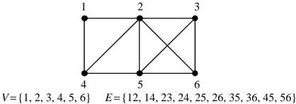
Let  $x, y \in V$ . An *x*-*y* path in *G* is a sequence of vertices starting with *x* and ending with *y*, in which each consecutive pair of vertices are adjacent. We require that all vertices other than *x* and *y* be distinct. If x = y, i.e. if the initial and terminal vertices in a path are identical, then the path is called a *cycle*. The *length* of a path is the number of edges traversed by the sequence. In the above example we have:
