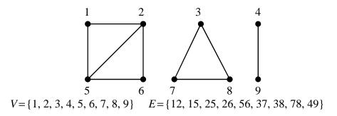
A subgraph of a graph *G* is a graph *H* in which  $V(H) \subseteq V(G)$ , and  $E(H) \subseteq E(G)$ . In the above example ({1, 2, 5}, {12, 15, 25}) is a connected subgraph, while ({2, 3, 6, 7}, {26, 37}) is a disconnected subgraph. A subgraph *H* is called a *connected component* of *G* if it is (i) connected, and (ii) maximal with
