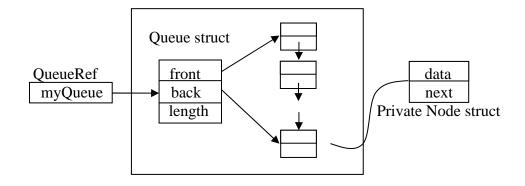
Two more C functions are necessary. One to create new objects (constructor) and one to free memory associated with ADT instances no longer in use (destructor). It is the responsibility of these functions to manage all of the memory inside the 'black box', balancing calls to malloc (or calloc) and free.
