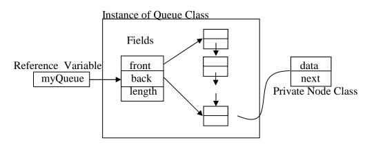
The user of the ADT should never be allowed to directly access the 'structure' inside the 'box'. Instead a reference variable (myQueue) points to an instance of the class and is passed as an (implicit) first argument to the methods of the class. For example, the call
