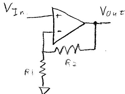
$$11 = \frac{V_{out}}{V_{in}} = 1 + \frac{R_2}{R_1}$$
