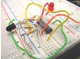
The proto-boards are fairly robust, however they are susceptible to damage from wires that are too large. Do not use hook-up wire larger than 24 gauge. This should not be a problem, since we are supplying hook-up wire kits. The other thing to watch for is component lead sizes. This will not be much of a problem during the labs, but you should be aware of these limitations since in later quarters you may use these boards to prototype your own circuits.
