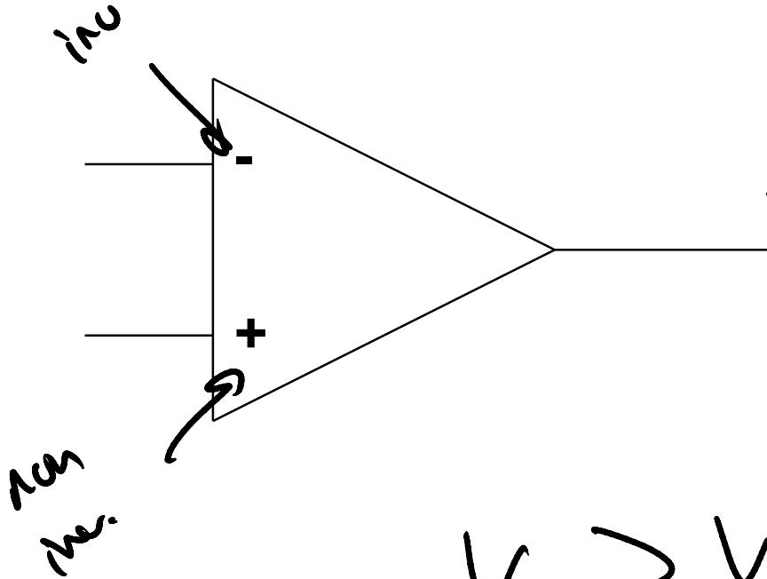
$$V_{out} = G (V_+ - V_-)$$
