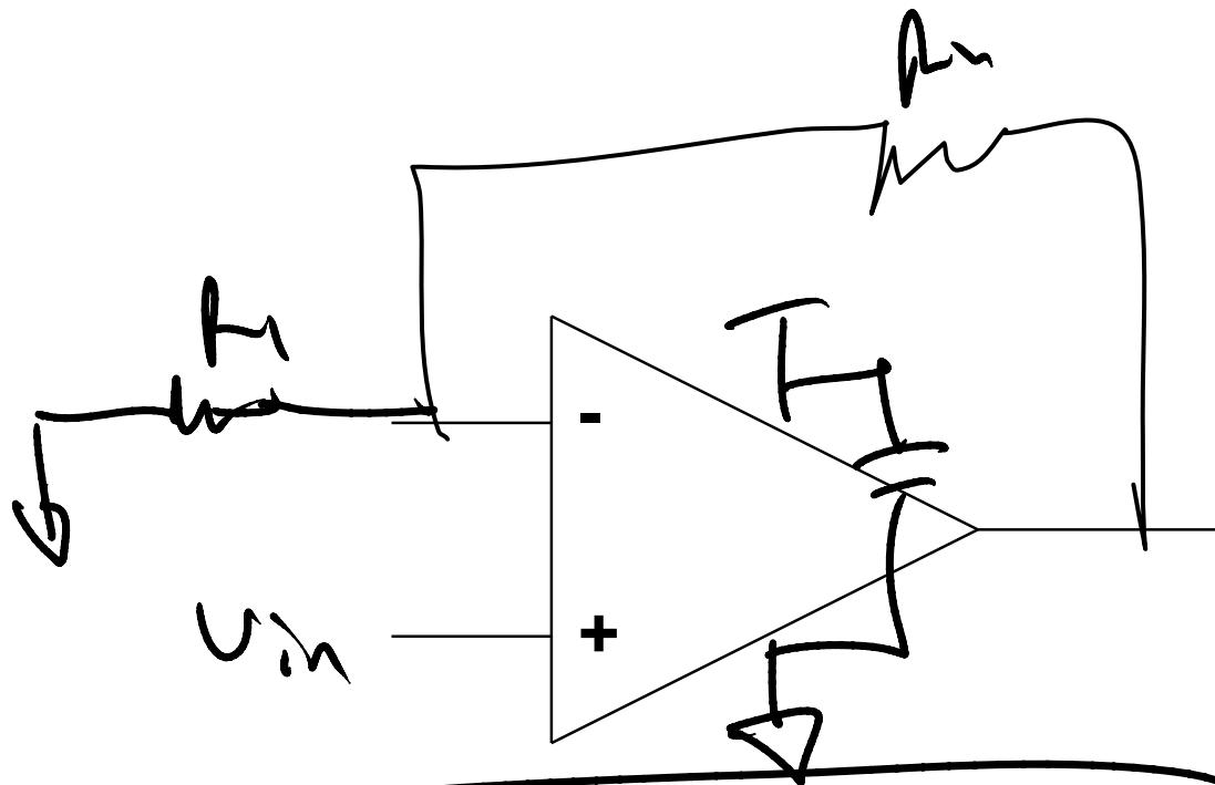
$$\frac{V_{out}}{V_{in}} = 1 + \frac{R_L}{R_1}$$
