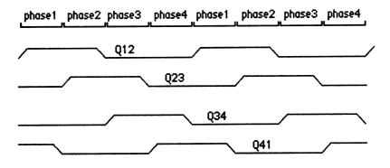
Note that Q12 and Q34 together form a non-overlapping two phase system, as do Q23 and Q41.
