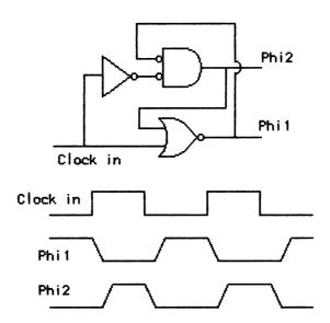
The non-overlap period must be long enough that all timing signals derived from the master clocks properly follow the two-phase discipline. There are several methods for ensuring this. The simplest is to make the
