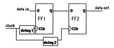
The figure shows a simple race condition. Two D flip-flops are connected in series to act as a shift register. When the clock line rises, data is supposed to be transferred from FF1 to FF2, and from the input to FF1. If the clock pulse arrives at FF2 sufficiently after it arrives at FF1, the input will be transferred to both FF1 and FF2. The difference in arrival time of supposedly simultaneous events is called *clock skew*.
